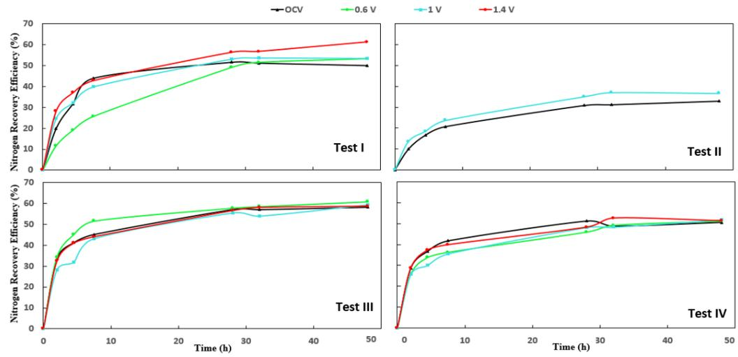
Figure 1. Nitrogen Removal efficiency at different voltage applied in four different situations: a) synthetic medium as anolyte and PBS as catholyte (Test I), b) synthetic medium as anolyte and NaCl as catholyte (Test II), c) pig slurry as anolyte and PBS as catholyte (Test III), d) pig slurry as anolyte and NaCl as catholyte (Test IV).
