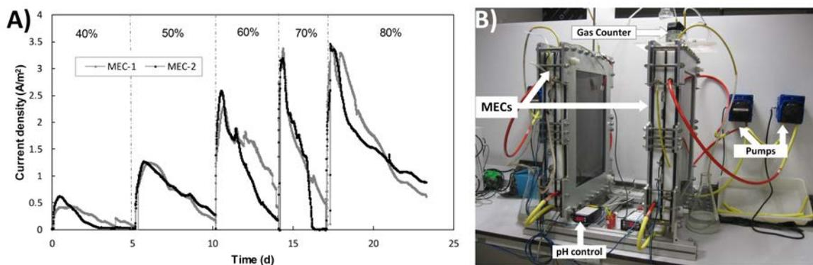
Figure 1. A) Current density (A/m<sup>2</sup>) at the different stages of the process (designated according to the percentage of slurry in the feed (40, 50, 60, 70 or 80%)) in MEC-1 and MEC-2. B) Reactor set-up.
